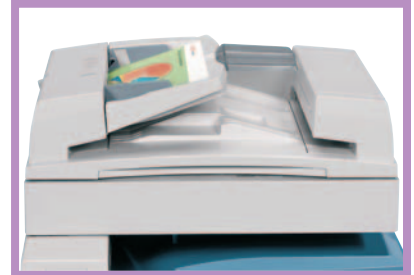
Duplexing Automatic Document Feeder (DADF-K1)
