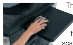
The cutting edge in biometric authentication, finger vein authentication uses images of finger vein patterns captured by scanning the finger. This
