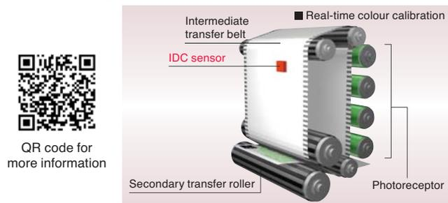
Konica Minolta's proven auto calibration system
