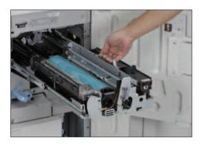
All three systems feature eight Trained Customer Replaceable Units (TCRUs), which trained operators can replace quickly and easily to maintain maximum uptime in certain environments.
