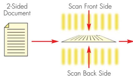
*Scan<sup>2</sup> Technology scans both sides of a document simultaneously, minimizing paper misfeeds dramatically.*
