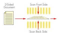
Scan<sup>2</sup> Technology scans both sides of a document simultaneously, minimizing paper misfeeds dramatically.
