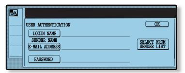
User Authentication requires users to log in to the machine before performing any network scanning operations, protecting it from unauthorized scanning and e-mail communications.
