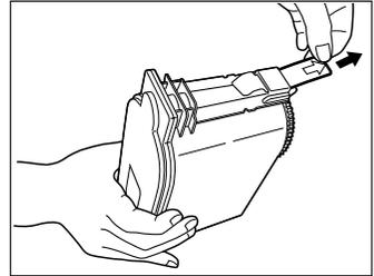
**5** Grasping the holder of the new toner cartridge, push it along the rail fully back into the copier.
