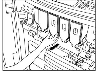
**3** Shake the new toner cartridge to the right and left 5 or 6 times to loosen the toner inside.
