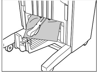
**6** Open the exit cover of the saddle stitcher and remove any misfed paper.
