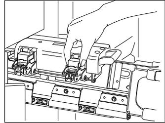
**3** While pushing down on the lever ①, pull up the knob ②.
