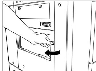
**3** Put down the lower guide of the exit side and remove any misfed paper.
