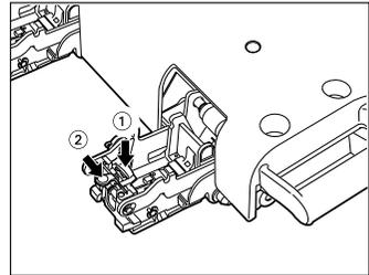
**4** Remove any jammed staples, and then return the knob ② to its original position.
