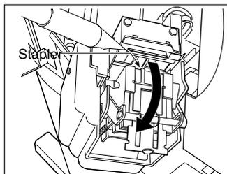
**4** Holding the knob, reinstall the staple guide in its previous position.
