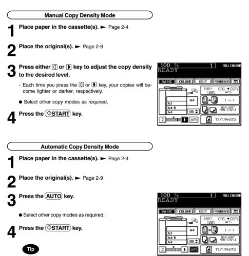
In the automatic copy density mode, the background level is detected during copying, so the copying speed becomes slower.
