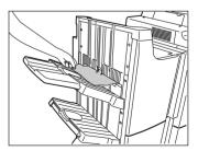
**f** Lift knob  $^{(1)}$  or knobs  $^{(1)}$  and  $^{(2)}$ , then remove any
