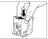
**8** Pull out the seal which holds the staples horizontally.
