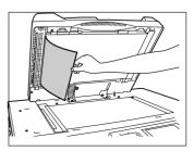
**3** Open the exit-side cover and remove any misfed originals.
