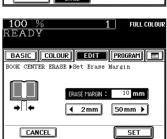
Utilizing this feature allows the facing pages of a book or magazine to be copied page by page onto two separate sheets of paper or duplex-copied on one sheet. There is no need to move the original on the glass. You can also place a pair of A4 (B5 or LT) sized originals side by side and copy them on separate sheets of paper.
