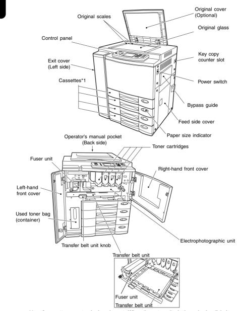
\*1.....2 cassettes are standard equipment. When the automatic duplexer (optional) is installed in the uppermost cassette, the 2nd to the 4th cassettes are for paper feeding (the 4th is an option).
