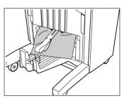
**6** Open the exit cover of the saddle stitcher and remove any misfed paper.
