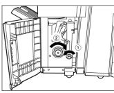
**5** Remove any paper misfed on the exit side of the saddle stitcher.
