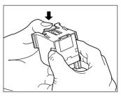
Push in a new staple case into the staple cartridge completely inside until a click is heard.
