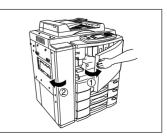
**2** Grasping the holder of the toner cartridge, slide the cartridge along the rail toward you and remove it.
